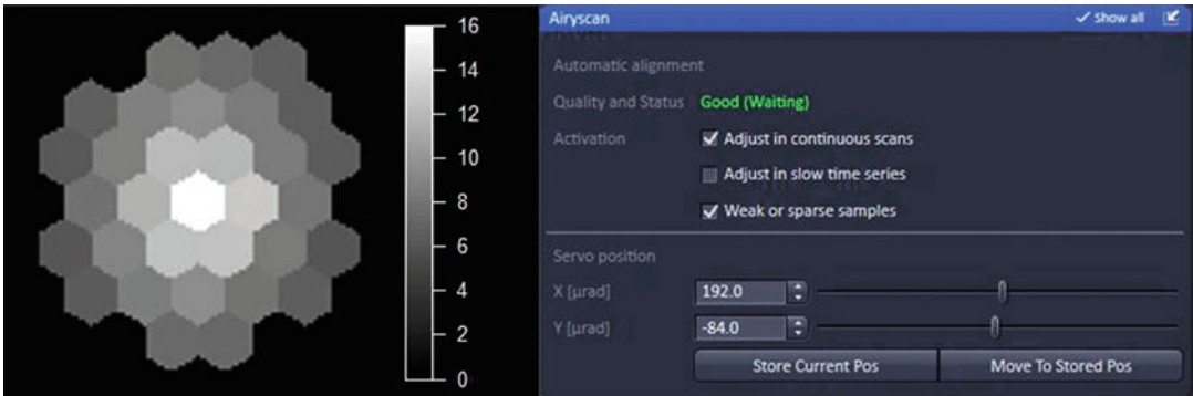
Fig. 3 Zen imaging software screenshot showing the Airyscan detector graphic and “maintain” tab indicating the quality and status of the detector alignment. The central detector on the Airyscan detector graphic should be the brightest when calibration is complete and the quality and status of the detector alignment should read “Good”
